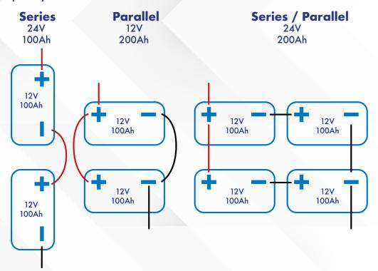
In any fitment where charging is via a dynamo or alternator, it is strongly advised to fit a DC-DC charger to control voltage. In systems that use a 'Smart Alternator' or where the voltage is above 15v for a 12v system or multiple's thereafter for series banks, a DC-DC charger MUST be fitted to avoid the BMS shutting down to protect the battery.
